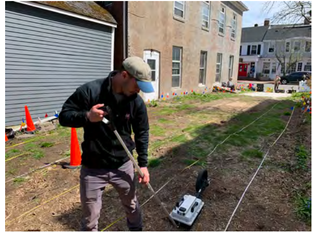
Figure 12a. Ground penetrating radar survey in the space between the Mansion and Brick Kitchen in progress.
